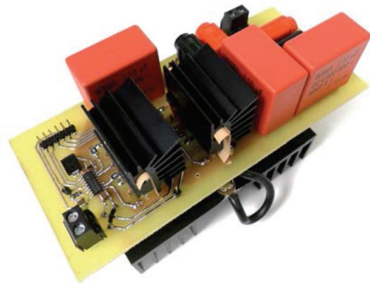
Figure 6.- Power inverter designed for these experiments
